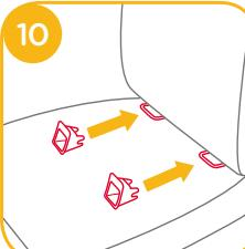
The ISOFIX guides can protect the surface of the vehicle seat from being torn. They can also guide the Isosafe connectors.
