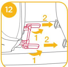
3. Line up the Isosafe connectors with the ISOFIX anchor points, and then click both Isosafe connectors into the ISOFIX anchor points. ⑬
