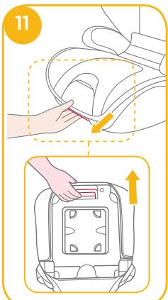
Rotate the Isosafe connectors 180 degrees until they are pointing in the direction of the ISOFIX guides.
