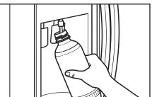
Rinse the carbonating bottle before use. Prior to making sparkling water, fill bottle with water up to the fill line. For best results, carbonate chilled water. To avoid product damage, carbonate water only.
