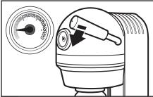
Carbonate in short pulses by pulling the carbonation lever down firmly and then allowing the lever to return to a middle rest position before repeating. Continue until the desired level of carbonation is achieved. Do not move the Sparkling Beverage Maker during the carbonation process.
