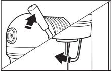
To insert bottle, make sure that the carbonation lever is in its fully upward position and the bottle loading lever is angled forward. If not angled forward, pull it toward you until it clicks. Do not pull carbonating tube.
