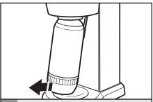
First remove the 1 L Carbonating bottle from the Sparkling Beverage Maker if you have already installed it.
