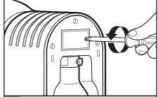
Use a Phillips screwdriver to loosen the screw holding the battery compartment cover plate in place.
