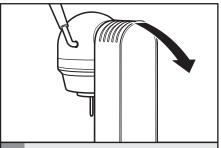
To remove back cover: Grasp back cover and pull away from unit. Set cover aside.
