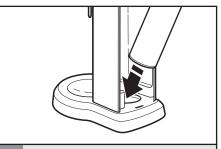
2 Remove seal and cap from SodaStream CO<sub>2</sub> Cylinder. Insert 60 L\* SodaStream CO<sub>2</sub> Cylinder into the Sparkling Beverage Maker. First tip downward into the base and then push upward into the valve fitting.
