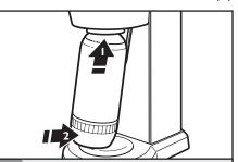
Insert bottle neck into the snap-lock. Firmly push bottle up and back. The snap-lock mechanism will catch the bottle firmly.
