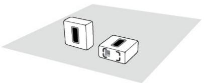
Make sure at least one side of the rectangular opening (acoustic slot) is unobstructed.
