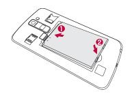
4 To replace the cover onto the device, align the back cover over the battery compartment and press it down until it clicks into place.
