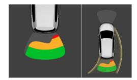
Depending on the vehicle and vehicle system it is also possible that the front PDC information is displayed.
