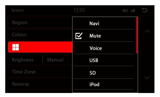
You can program the button to allow instant access to many features. choose the function or mode that will be instantly accessed on the press of the button like navigation, Multimedia or even the reverse camera mode.
