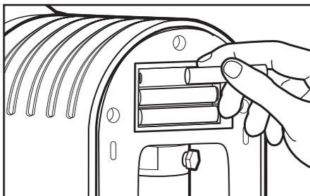
**3** Replace three AAA batteries in the battery compartment, put the cover plate in place and secure with the screw.
