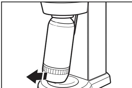
**6** Pull bottle toward you to release bottle from snap-lock; the bottle will be released automatically.
