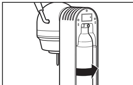
**3** Turn the SodaStream CO<sub>2</sub> Cylinder counterclockwise until it stops. Hand-tighten only.
