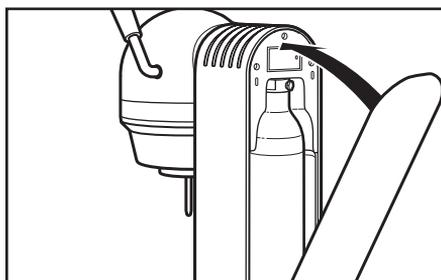
**4** To reinstall back cover: tilt back cover toward you; insert bottom tab into slot and push cover into place.
