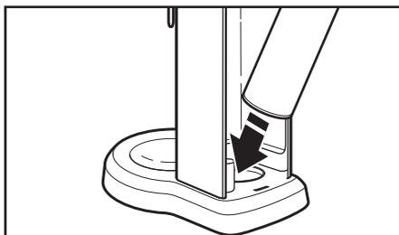
**2** Remove seal and cap from SodaStream CO<sub>2</sub> Cylinder. Insert 60 L\* SodaStream CO<sub>2</sub> Cylinder into the Sparkling Beverage Maker. First tip downward into the base and then push upward into the valve fitting.
