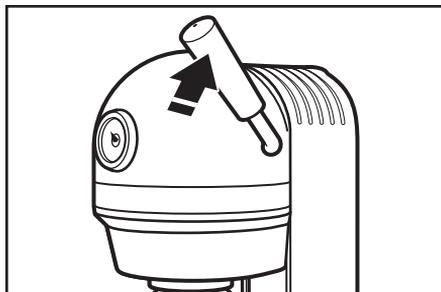
**5** To release bottle, push Carbonation lever to its fully upward position. You will hear the sound of excess CO<sub>2</sub> discharge.
