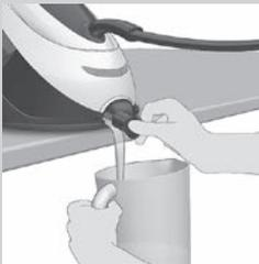
**4** Remove the EASY DE-CALC knob and let the water with scale particles flow into the cup.
