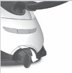
**5** When no more water comes out of the appliance, reinsert the EASY DE-CALC knob and turn it clockwise to fasten it.
