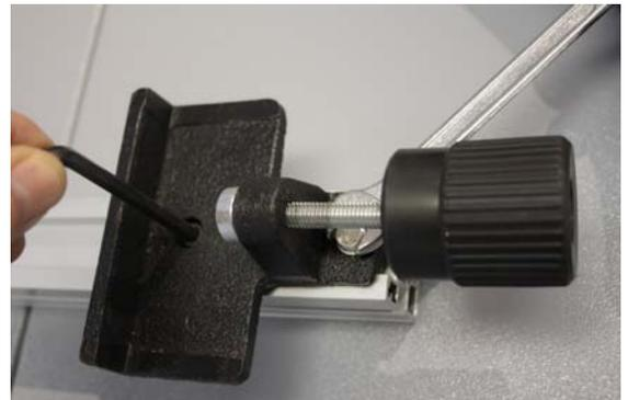
Screw the adapter as shown on the aluminum profile and slide it into the rip fence guide profile.
