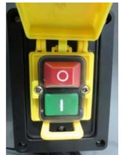
**INFO:** In the closed state of the main switch can be operated as an **EMERGENCY STOP** switch.
