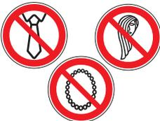
When working with the machine, do not wear loose jewelry, wide or protruding from the body of clothing, ties, long hair out, etc.
