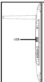
USB data carriers can only be plugged into the USB slot in one direction.
