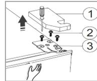
Loosen the screws (2) and remove the upper door hinge (3).
