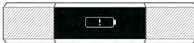
Critically low battery
