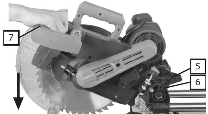
Turn the table (20) until the mitre angle indicator points to 0°. Tighten the mitre angle lock.
