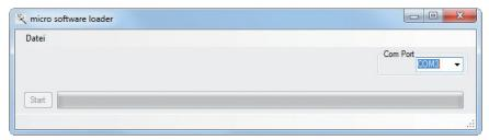
If you are not sure which port to use, check the COM port in the "Select Port" window in the "Menu" of the "Firmware\_Up-grade\_grStudio" and note down the COM port number for the "Silicon Labs CP210x USB to UART Bridge" entry—in this case "COM03". (If you select the wrong port, you will be alerted to this when you read out the receiver data). Click on "File" to load the corresponding firmware file named "MicroStabi7X\_V\_XX.bin" from the hard disc ("XX" stands for the version number).
