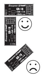
The receiver must be aligned at right angles to the copter on the receiver platform. The lower surface of the receiver must always be parallel to one of the copter sides. Prior to installation, remove the sticker on the back of the receiver. We recommend using double-sided tape No.: S8376 for Gr-18 to fix the receiver in place.
