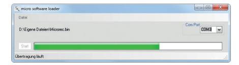
The progress bar shows that the transfer is running normally. The receiver LED lights up red and green during this process and flashes red and green alternately once the transfer is complete.
