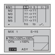
In Acro 3D Mode: In addition to the motors stop switch you need to program a mixer to be able to switch the motors off in 3D Acro mode too. If the 3D Acro mode enabled and you control over the rate mode, the motor stop function would control the motors fully backward. To prevent this, the mixer switches to attitude mode, here then the stopping of the motors is ensured via the switch. Set a free mixer from S1 to CH5. (see display screenshot on the left)
