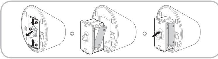
1. Hold the both sides of the battery holder and pull it out.
