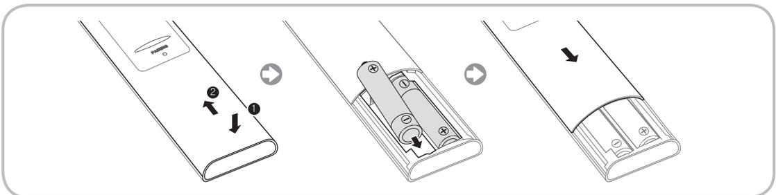
1. Press the back of the remote at the very bottom with both thumbs, and then slide the battery cover up in the direction of the arrow.
