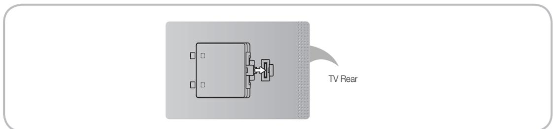
This socket is designed to accept an extension device called Evolution Kit. The Evolution Kit enables the TV to run a variety of the latest applications for a better user experience.
