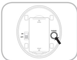
1. Turn on the IR Blaster. When Indicator LED blinks, you should connect IR Blaster to TV.
