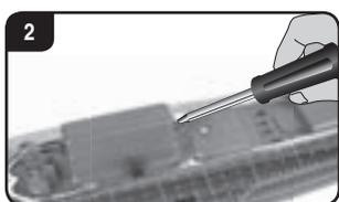
Using a screwdriver, remove the cover of the battery compartment in the Carrera RC boat.
