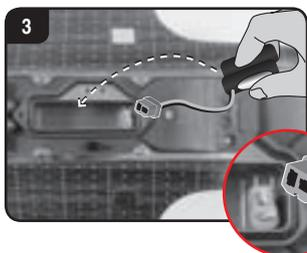
Connect the end of the cable from the Carrera RC boat with the charged battery. Put the battery in place. Replace the compartment cover using a screwdriver.
