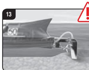
**Be sure not to allow the propeller or the rudder to touch the bed of the water.**
