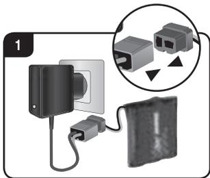
First connect the Carrera RC rechargeable battery to the battery charger supplied. The connection terminals between the battery and the charger are designed to prevent connection with the wrong polarity. Connect the charger to a power source.
