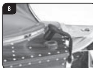
After each running session, open the drainage plug at the stern and pour away through this opening any condensation which may have accumulated. Only replace the drainage plug in the opening provided immediately before you use the boat for another running session.
