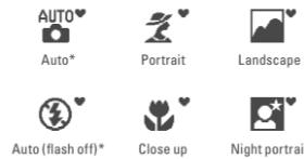
If you are taking still pictures using D3200's "live view" monitor and are using the Auto or Auto (flash off) functions, the Scene Auto Selector\*\* can automatically select the most appropriate set-up from a choice of options: Portrait, Landscape, Close up and Night portrait. The D3200 self-configures to ensure optimum results, leaving you more time to concentrate on composition.
