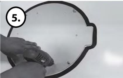
Put back the mounting plate on the silicone applied and make 6 holes (2mm).
