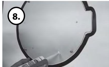
Re-apply silicone to cover bolts assembled
