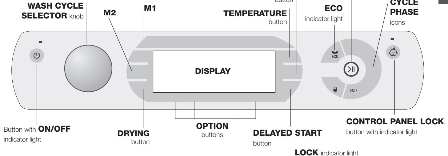
**Button with ON/OFF indicator light:** press this briefly to switch the machine on or off. The green indicator light indicates that the machine is switched on. To switch off the Washer-dryer during the wash cycle, press and hold the button for approximately 3 seconds; if the button is pressed briefly or accidentally the machine will not switch off. If the machine is switched off during a wash cycle, this wash cycle will be cancelled.
