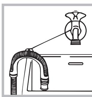
Alternatively, rest the drain hose on the side of a washbasin or bathtub, fastening the duct supplied to the tap (see figure). The free end of the hose should not be underwater.
