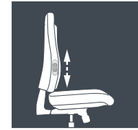
Backrest with integrated height adjustable lumbar support
