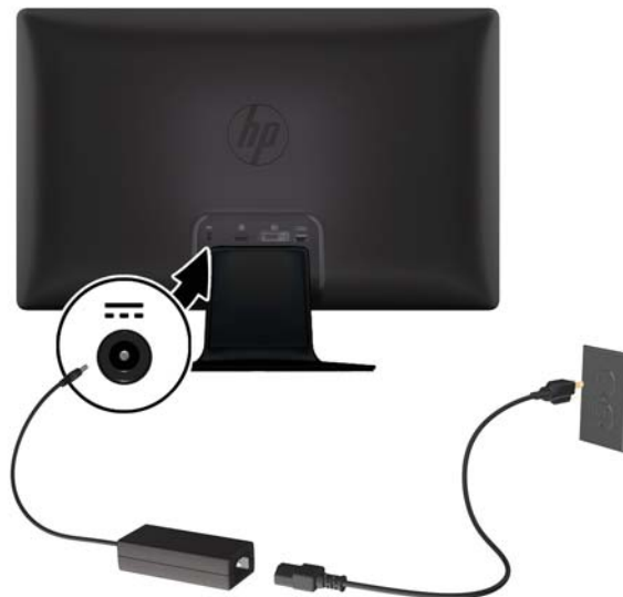
Figure 3-6 Connecting the Power Cord
