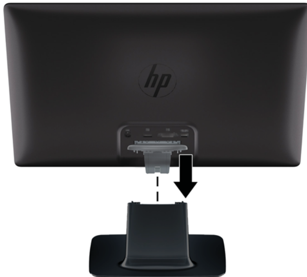
Figure 3-2 Inserting the Monitor Panel
