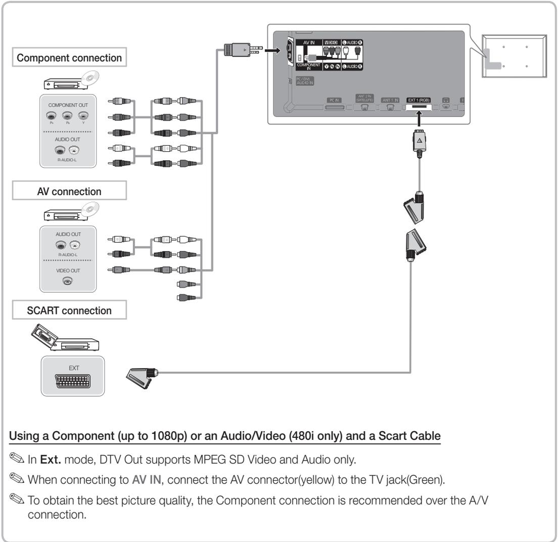
**Using a Component (up to 1080p) or an Audio/Video (480i only) and a Scart Cable**
