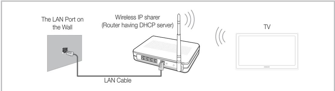
Samsung's Wireless LAN adapter supports the IEEE 802.11a/b/g and n communication protocols. Samsung recommends using IEEE 802.11n. When you play the video over a IEEE 802.11b/g connection, the video may not play smoothly.
