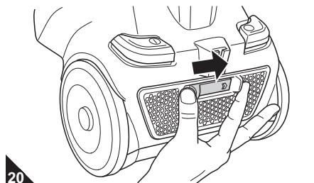
3. Remove the exhaust filter.
