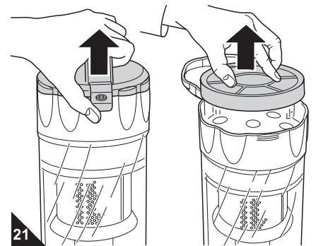
3. Hold the dual motor protection filter deep inside a dustbin and only then separate the filter elements from each other.
