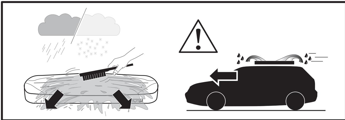
**GB** Attention: Water/snow accumulation on unloaded box. Secure that the contents of water/snow is emptied before travelling.
