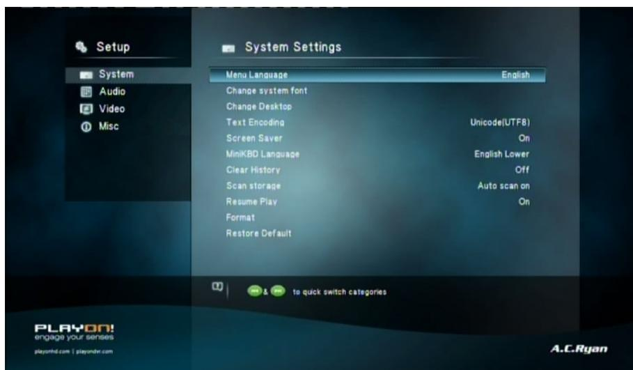
There are four Setup options, including **System**, **Audio**, **Video**, and **MISC**. Use the **UP/DOWN** navigational buttons to select a menu. Press **ENTER** to confirm. Press **RETURN** to cancel and display the previous menu screen.
