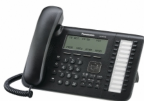
KX-NT546 - Standard IP Phone with 6 line Display
